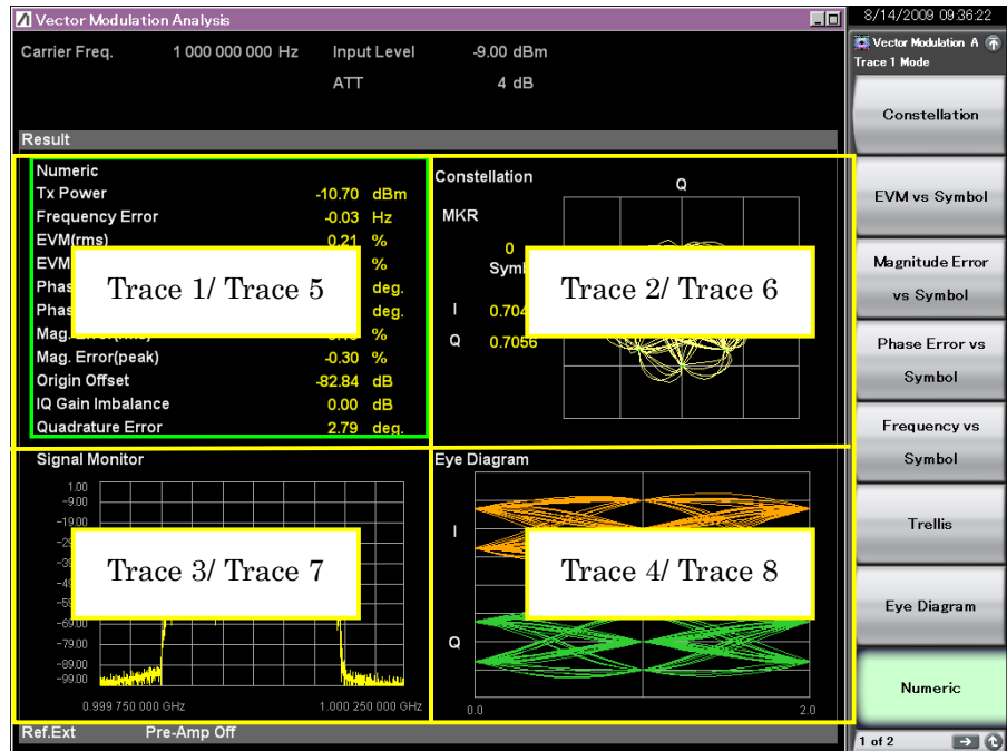
Figure 3.1.1-2 Trace Window (4-Split Screen)
